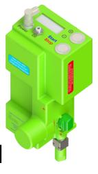
All smartTensioner devices operate with silicon oil as hydraulic medium. Oil with extremely high viscosity is needed to allow small and powerful tensioning devices. While other commercially available pumps are not able to pump these kinds of media, smartTensioner HP has been designed for this very objective.
